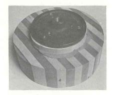
7. Always revolve the workpiece by hand before turning on the motor to make sure that it does not strike the tool rest.
