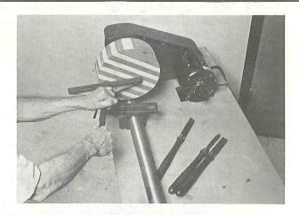
6. As the inside of the workpiece approaches the finished contour, use the Bowl Turning Tool Rest. IMPORTANT . . . set it 1/8 inch below center and adjust the stop collar.
